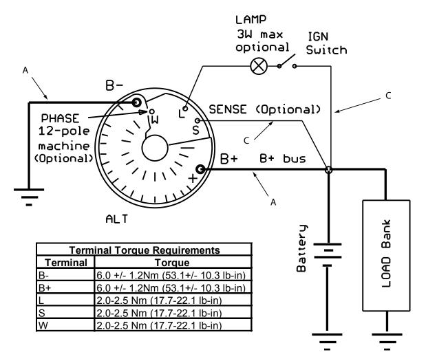
For A and C wire requirements, see TSB-1001 for wire gauge sizes.
